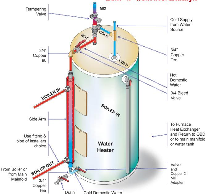
Water -to- Water Heat Exchanger Side Arm Assembly Parts List
